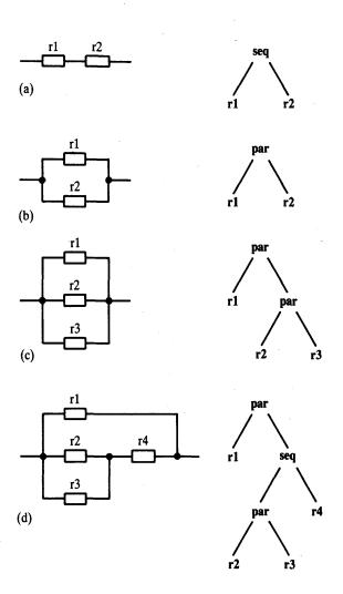
**Figure 2.6** Some simple electric circuits and their tree representations: (a) sequential composition of resistors r1 and r2; (b) parallel composition of two resistors; (c) parallel composition of three resistors; (d) parallel composition of r1 and another circuit.
