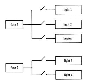
Figure 14.6 Connections between fuses and devices in a simple electric network.
